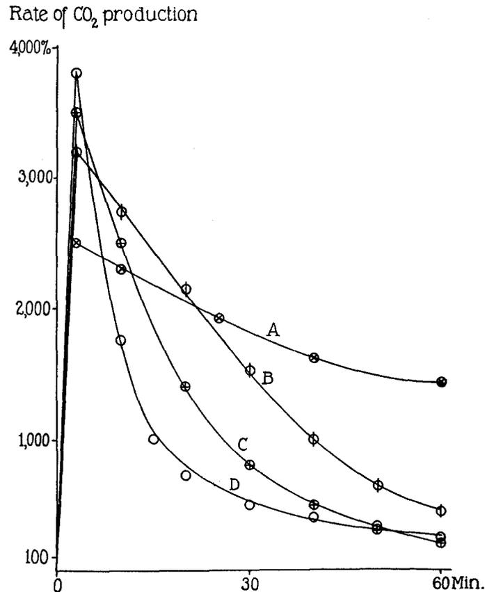
FIG. 1. Curves showing the rate of production of CO<sub>2</sub> by a solution of dextrose and hydrogen peroxide. Curve A shows the rate in a solution having a pH of 8.75, B in a solution of pH 7, C in a solution of pH 5, D in a solution of pH 1. The rate in the absence of hydrogen peroxide is taken as 100 per cent.
