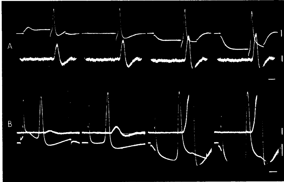
FIGURE 7. Effect of polarization of presynaptic axon on the p.s.p. and on the presynaptic action potential. A , recorded at synaptic region; upper beam, presynaptic action potential. Lower beam, p.s.p. B , recorded at a point about 2 mm proximal to synaptic region; upper beam, p.s.p.; lower beam, presynaptic action potential. Time scale, 5 msec. for A , 2 msec. for B . Voltage scale, A upper, 20 mv; A lower, 1 mv; B upper, 5 mv; B lower, 20 mv.
